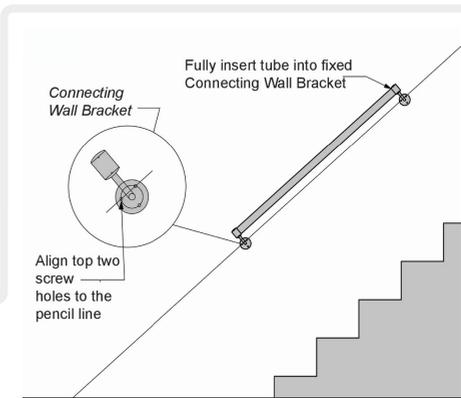
Drill Ø8mm diameter holes for the wall plugs being used, insert wall plugs and using screws provided, screw the Connecting Wall Bracket to the wall. Tighten the two tube retaining screws at either end holding the tube in place using the allen key provided, ensuring you do not over tighten.
