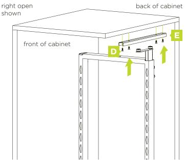
Align the U-Iron (E) with the pre-drilled holes and using 4 x 16mm wood screws (D), fix the U-Iron to the top of the cabinet.
