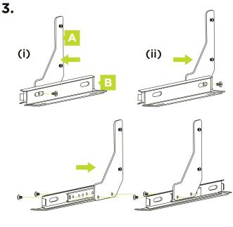
Remove two flat head screws from each L-Iron (A) and attach to the runners (B) as pictured above. **NOTE:** You will need to slide the runner forward (i) and backward (ii) to access the round holes of the runners. Be sure to screw through the runner to the L-Iron as above.
