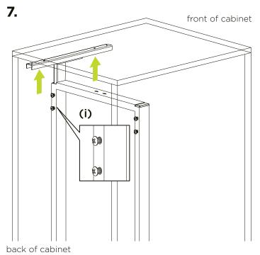
Loosen the 2 screws at the back of the frame (i). Adjust the L-Bracket up so the castors are slotted into the U-Iron completely and tighten screws (i).
