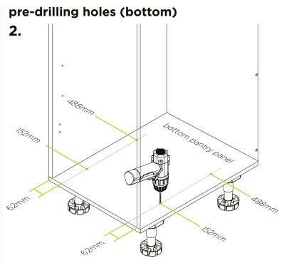
Mark out and pre-drill four holes on the bottom panty panel as per the diagram above. Use a 2mm drill bit to pre-drill holes to a depth of 2.5mm.
