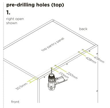
Mark out and pre-drill four holes on the top panty panel as per the diagram above. Use a 2mm drill bit to pre-drill holes to a depth of 2.5mm.
