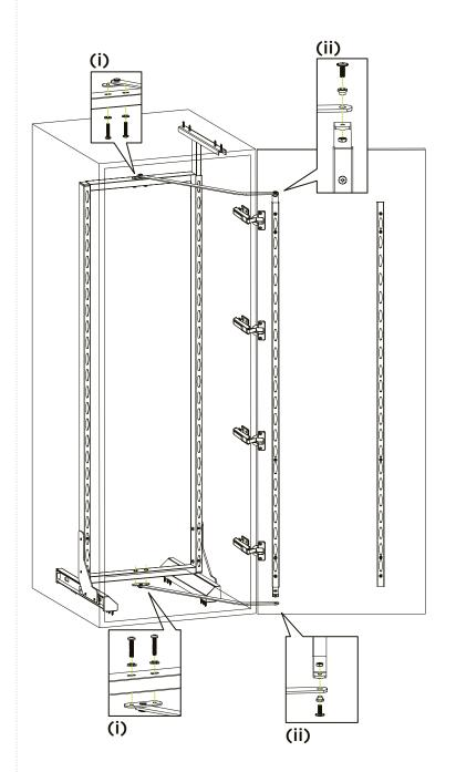
Attach the door to the cabinet. **NOTE:** If not a retro-fit installation you will need to install your hinges at this point.
