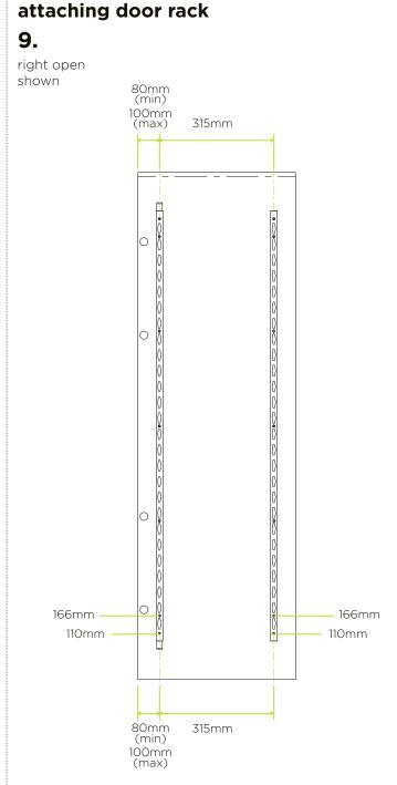
On the back of your pantry door, draw a level line the length of the door 80-100mm from the inside edge. Next draw a second line the length of the door 315mm over from the first line.
