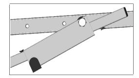
The smaller Addaline frame is raised by manually securing the wire Braces into the Side Arm's larger punched holes. To lower the frame, hold the front bar and remove each wire Brace from the Side Arm hole. Carefully lower frame.
