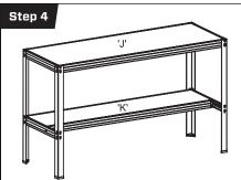
Place bottom MDF shelf 'K' onto bottom braces and top MDF shelf 'J' onto top braces ensuring both shelves sit flush.
