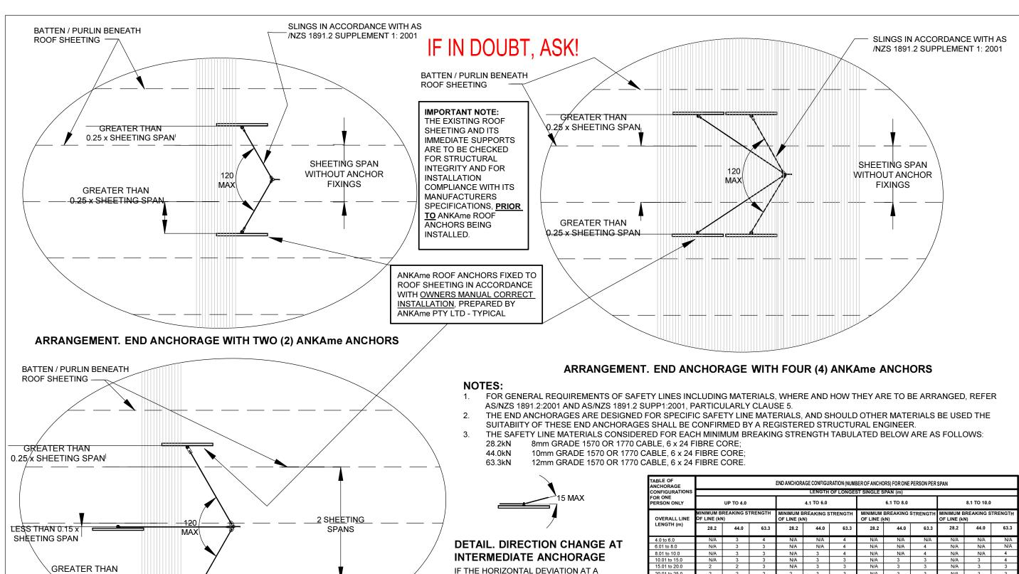
IF THE HORIZONTAL DEVIATION AT A POTENTIAL INTERMEDIATE ANCHORAGE IS GREATER THAN 15° THE LINE SHALL BE TERMINATED AND RESTARTED AT THAT POINT WITH A SEPARATE SET OF END ANCHORAGES AS CONFIGURED ABOVE. EACH SEPARATE LINE IS TO HAVE ITS OWN ANCHORAGE SYSTEM AT EACH END. ROOF ANCHORS TO BE FIXED TO THE ROOF SHEETING NORMAL TO ITS RIB DIRECTION.
