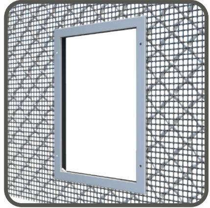
Fit all four partitions into outer door frame, use duct tape to secure the corners then place into opening. If the security screen has insect mesh, place a bead of construction silicon around the internal section of the pet door and on the mesh surface. Apply this around the cut out in order to hold the mesh in place when both frames are joined.
