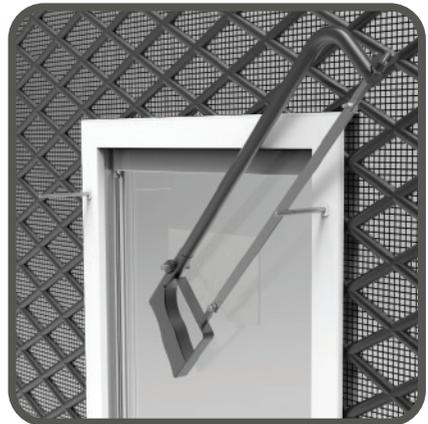
Screw inner door frame into door/panel. Tighten with a Phillips headscrew driver. If screws protrude, trim using a hacksaw.
