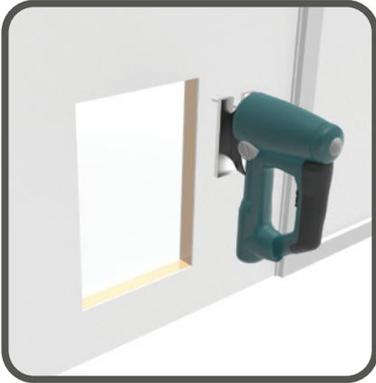
Using a reciprocating jigsaw, cut out the opening, cutting along the pencil outline.
