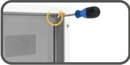
1. Loosen screws on flap holder.
