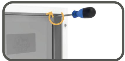
4. Tighten flap holder screws.
