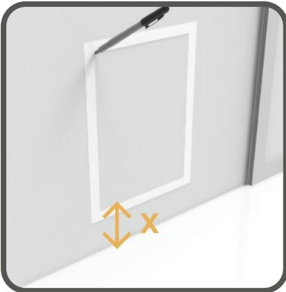
Cut out template supplied in box, align bottom of cut out with height (x) and trace onto door.
