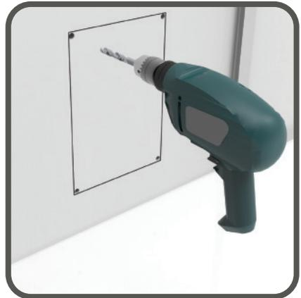
Drill a hole in each of the four inside corners with a minimum of 10mm (3/8") drill bit.
