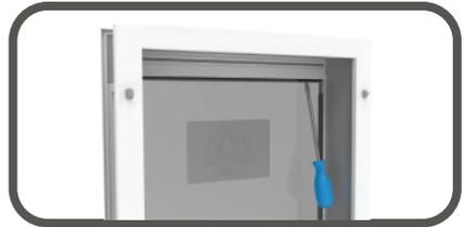
2. Use a flat blade screwdriver to pry open the flap holder.
