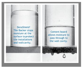
The test demonstrates DensShield Tile Backer stops water at the surface, while cement boards allow water to pass through their porous construction. The Tile Council of North America requires the use of a membrane in wet areas for cement backer boards but does not require a membrane for DensShield Tile Backer since DensShield Tile Backer panels have a built-in moisture barrier that stops moisture at the surface.
