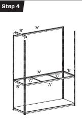
Place 1x MDF Shelf on the bottom brackets to minimise buckling. Fix brackets 'A' and 'B' at the very top of the leg uprights, then repeat with other brackets at your desired heights.
