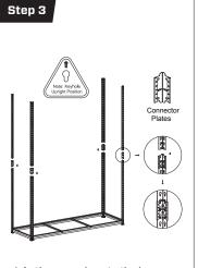
Join the upper leas to the lower legs with the connector plates.
