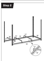
Use shelf bracket 'B' for the side brackets using the shelf bracket from Step 1 as a guide for height. Use same shelving brackets for opposing sides as shown in the
