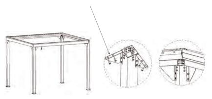
NOTE: Make sure all 4 posts are level as the gutters are a snug fit. You may be required to loosen bolts for brackets in order to fit gutters. If you do, remember to re-tighten before continuing.
