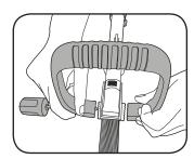
2. Place the adjustable handle on the mounting bracket, then pass the screw with washer through the handle and onto the mounting bracket.
