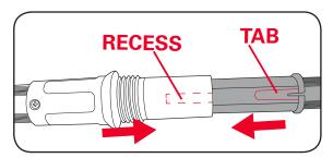
2. Screw tight with the shaft lock collar.
