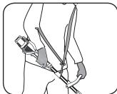
3. To turn on squeeze the variable speed trigger whilst holding the safety switch forward.
