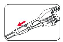
Squeeze the variable speed trigger to start the line trimmer.
