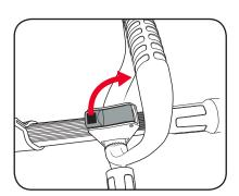
2. Slide the handle into the desired position and then lock in place with the lever.
