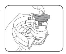
4. In case of jams and tangled line, unwrap about 15cm of line to ensure that it is undamaged. If it is OK, thread the end of the line spool through the eyelet in the spool cover
