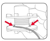
To ensure that the line does not unravel while the spool is being loaded, the line can be clipped into one of the notches on the outer of the spool.
