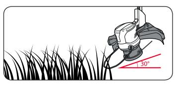
Use only the tip of the cutting line to do the trimming especially near walls and fences. Trimming with the side of the cutting line may overload the motor, wear out the line faster, and break the line more often.
