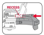
3. Slide the safety guard in place and secure with the socket head bolt. Tighten with the hex key.
