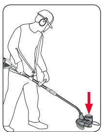
CAUTION: DO NOT BUMP THE HEAD ON ANY HARD SURFACES SUCH AS CONCRETE OR BRICK, THIS COULD CAUSE DAMAGE TO THE LINE TRIMMER.
