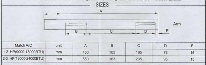
Note: 1. Ensure that the wall bracket is mounted properly to handle applied loads as wall construction may vary.
