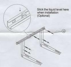
PS: Please check and make sure connecting screws should be tightened on the bracket after finished installation
