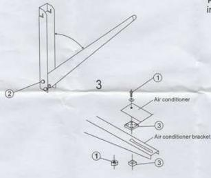
Fix bracket to the wall using the holes provided in the bracket to complete installation.
