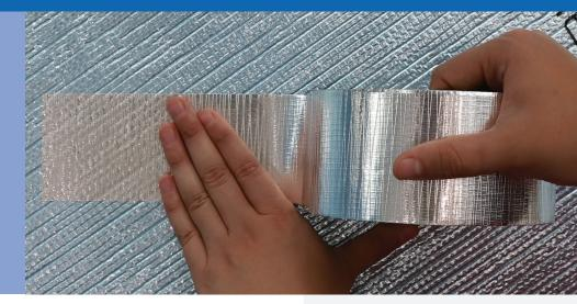
Ametalin Reinforced Insulation/Ducting Tape is a high performance 0.178 mm UV-resistant PE scrim reinforced tape coated with a cold weather acrylic adhesive. Designed with vapour-sealing properties to complement our full range of reflective membranes, it can be used with all roof sarking, wall wraps and floor insulation. It is also ideal for use in the HVAC and ducting industry.
