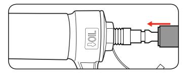
ENSURE THAT THE COMPRESSOR PRESSURE DOES NOT EXCEED 120PSI.
