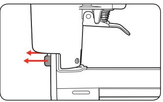
2. Remove the front plate held by the two screws.
