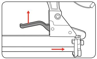
2. Place a row of staples into the middle of the magazine so that the staples fit cumfortably in the inner chamber.
