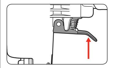
**Note:** The stapler will only fire once if the trigger is held up. The trigger must be released to fire a second staple.
