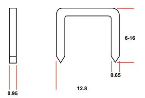
Note: All measurements are in mm.
