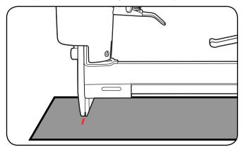
2. Push the tool firmly down on the work surface.
