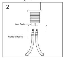
Firmly tighten the flexible hoses into the inlets, being careful to avoid damage to the O-ring seals. If the hoses have red and blue indicators make sure they are connected to the correct inlet ports in the mixer.
