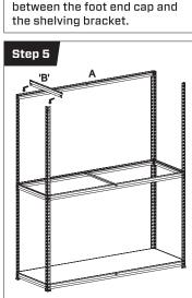
Fix brackets 'B' at the very top allowing room for the MDF board to sit flush against the legs. Repeat with brackets 'A'.
