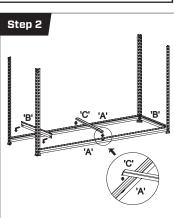
Use shelf bracket 'B' for the side brackets using the shelf bracket from Step 1 as a guide for height. Allow one keyhole free from the ground as shown in the diagram. Use same shelving brackets for opposing sides as shown in the diagram. Place bracket 'C' as shown.
