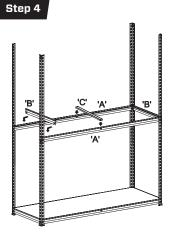
Fix brackets 'B' so that the top rivet sits on the upper legs and the bottom rivets sit on the lower legs. Repeat with brackets 'A', followed by brace 'C' as shown.
