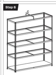
Apply remaining brackets as above to desired height. Ensure that braces 'C' are fixed to all shelves. COATED BLACK PER SHELF
