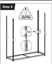
Place MDF board on bottom shelf to minimise buckling. Join the upper legs to the lower legs with the connector pins. Note upright position. Note: The legs are designed to sit directly on top of each other don't overlap them. Handy Hint: Flathead screwdriver may be used to tap in connector pins.
