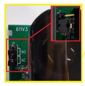
The GTR196 comes with a moveable jumper pin. This allows a Normally Open (N.O) or Normally Closed (N.C) function.
