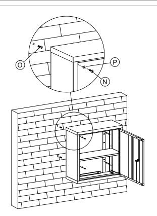
Alternatively, the cabinet can be mounted onto a wall. First drill four holes which align exactly with the holes on the back panel (D) for mounting the cabinet. Then insert the included plugs (O) into the drilled holes and use the long self tapping screws (N) and washers (P) to fix the cabinet to a wall.
