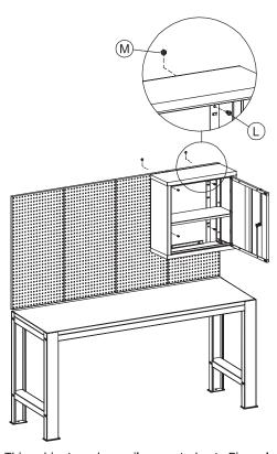
This cabinet can be easily mounted onto Pinnacle Hardware's pegboard (Model number: GOSO83) using the provided Phillips head bolts (L) and hex nuts (M) as shown in the diagram above.
