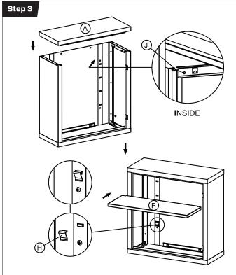
Place top panel (A) onto the pack panel (D) and side panels (B & C) and gently push down to engage the tabs into the slots on the back and side panels. Once tabs have been inserted, fix all panels together using the provided self tapping screws (J) as per diagram above. Insert the shelf supports (H) into the slots in all four corners at an even height and insert shelf (F).
