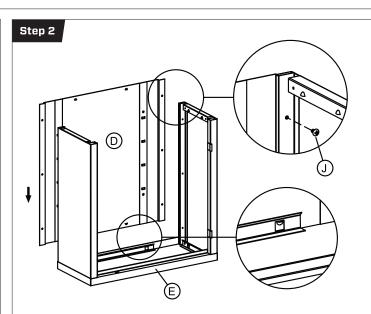
Once left and right side panels (B & C) are fixed to the bottom panel (E) slide the back panel (D) into the bottom panel (E) ensuring the tabs on the back panel (D) insert into the slots on the bottom panel (E). When back panel (D) is in place, fix to side panels (B & C) using the provided self tapping screws (J) as per diagram above.
