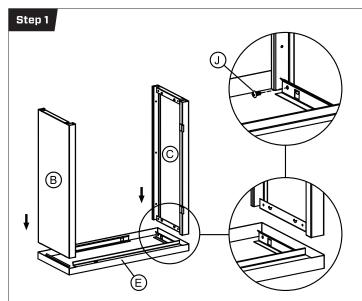
Slide left side panel (B) into bottom panel (E) making sure the tabs insert neatly into the slots on the bottom panel (E) as per the diagram above. Fix left side panel (B) using two of the provided self tapping screws (J) as per the diagram. Now repeat the same process for the right side panel (C).
