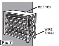
Fit 2 Long Top Support Single Rivet Beams and 6 2 Short Top Support Single Rivet Beams to the top two holes of the Keyhole Uprights. (Pic 6) **IMPORTANT:** Only use Long and Short Top Support Beams for Top Shelf position.
