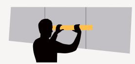
Note: Alter the thickness of silicone applied behind the different sizes of glass and polymer to obtain a flush finish across all materials.
