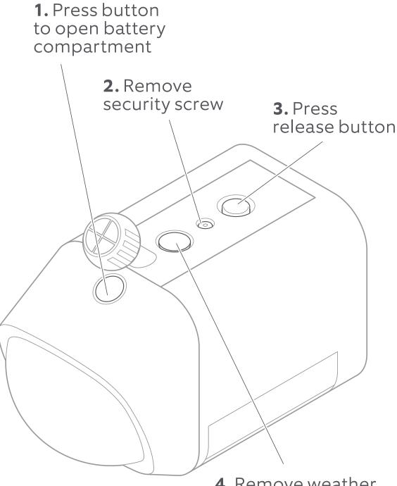
**4.** Remove weather seal, and insert in unused hole
