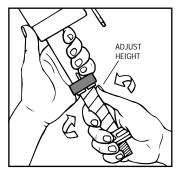
3. To adjust valve height, remove it from cistern. Twist threaded shank in or out of valve body without moving grey ring (height adjusts from 225mm. to 350mm. – the clicking noise heard is normal). NOTE: Adjust height so that the critical level mark (marked "C.L.") on the valve body is at least 25mm. ABOVE the overflow outlet in the cistern.
