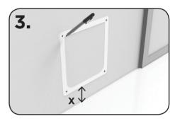
3. Cut out supplied template, line up height (x) with opening & trace on to door.
