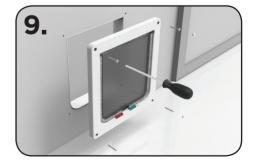
9. Screw into door from both sides and cover screws with screw covers.
