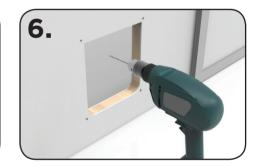
6. Check outer frame fits opening and screw holes align. Drill 3mm (3/32") pilot holes.
