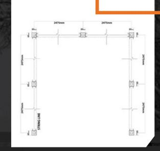
// Make up each of your posts according to step 1 using the 65mm x 65mm square posts and the Panel Channel. Each post is made according to its position in the layout and is either a 180 degree, 90 degree or an end-of-line combination.
