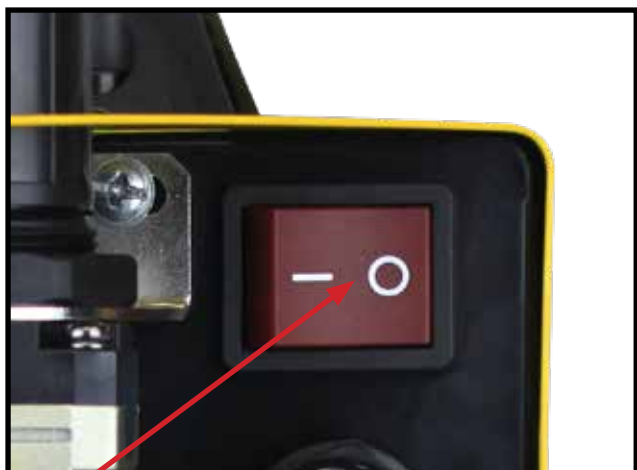
2 Plug the machine input power lead into the 15 Amps wall socket, ensuring that the Mains Power Switch is OFF.
