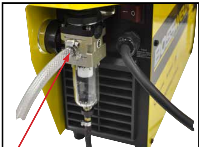
1 Install the compressed air hose to the connector at the rear panel of the machine to the Compressed Air Inlet.
