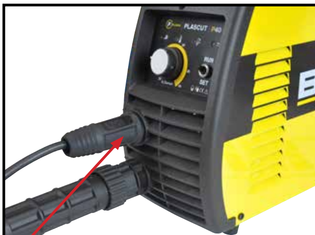
4 Connect the earth lead to the Earth Lead Connection Socket (positive) and connect earth clamp to work piece ensuring that the clamp makes good contact with bare metal.
