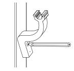
**3.** Drill a 6.5 mm hole through the balustrade post at the marked position.
