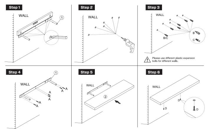
Please note: For safety, the bracket pipes are angled slightly upward to prevent shelf droop when shelf is loaded to capacity.
