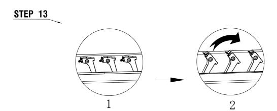
Before installing the shutter (F), use the handle (R) to rotate the louvre arms from position 1 to position 2 (as pictured above).
