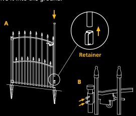
A: Slide retainer onto second post and insert post down into spike. Then secure with pin (provided).
