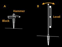
A: Position the first spike and hammer it into the ground until the top of the blades are flush with the surface.
