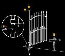
A: Insert first post through the gate hinges and down into the spike. Then secure with pin (provided).
