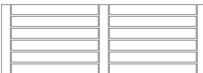
Example of a breaker board design (recommended for decks longer than 5.4m):
