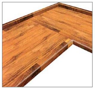
Fig. 17 Butt joint
