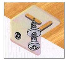
Fig. 16 Do not over tighten screws
