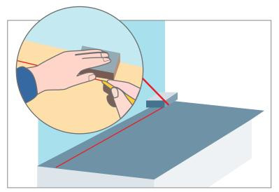
Fig. 6 Scribing to correct depth
