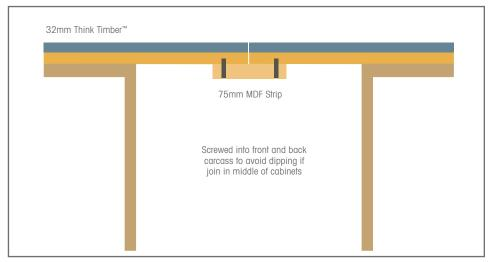
Fig. 5 (not advisable) Join in middle of unit with MDF strip (if recommended position not possible)
