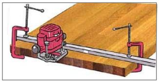
Fig. 13 Standard cut method with router
