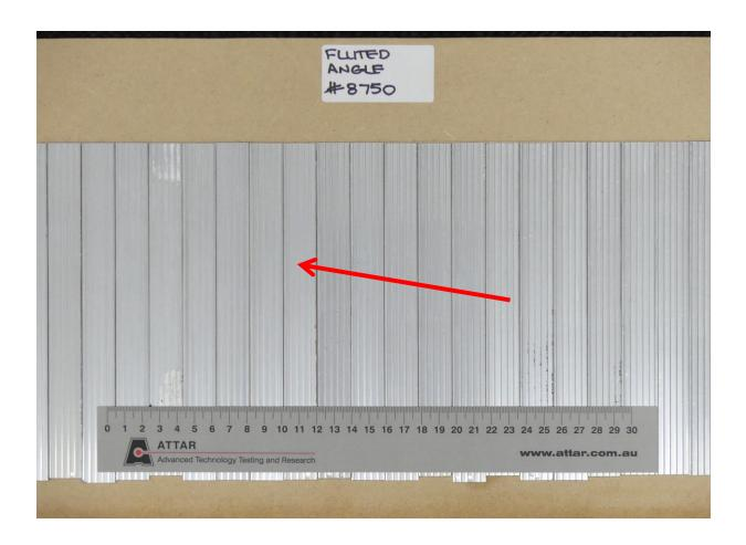
Figure 1: Fluted Angle #8750 stair nosing Arrow indicates direction of testing
