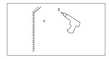
3. Drill 6mm diameter holes into the marked out location. Note - use appropriate drill bit(ie - masonry bit for tiles). Check wall plugs provided for accurate measurements.
