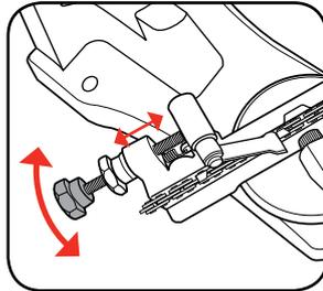
3. When the chain stop is properly adjusted it should be directly behind the chain tooth as shown. To secure in position rotate the lock knob clockwise as far as possible.
