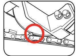
Alternatively, you can lower the wheel until it firmly sits on top of the tooth body and then rotate the depth adjustment knob 1/2 a turn clockwise to lift it slightly away from the body. Lifting the wheel away from the body will prevent cutting into the body or link and damaging the chain.
