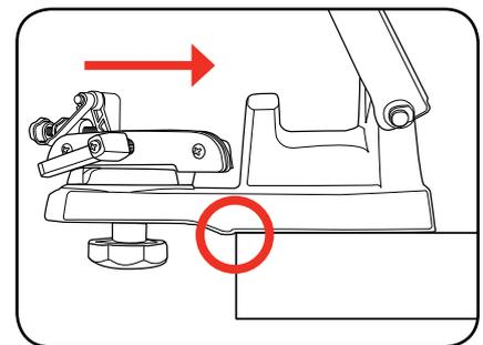
Two 6mm mounting holes allow for fixing the base to the mounting surface (bolts not supplied). Ensure the mounting surface is capable of supporting the weight of the sharpener and chain to be sharpened.
