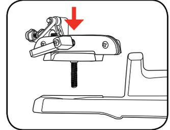
2. Secure the table in place by fixing the locking knob to the bolt (by screwing the knob clockwise).
