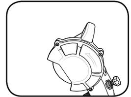
4. Lower wheel towards the face of the tooth. The depth pin should meet the depth stop platform and stop the wheel from travelling the full distance to the tooth.
