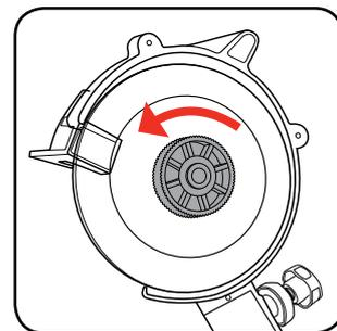
5. Remove the wheel and replace with a new one.
