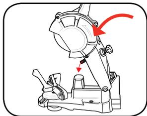
**CAUTION:** DURING OPERATION, IT IS IMPORTANT NOT TO OVERLOAD THE SHARPENER. THE SHARPENER SHOULD RUN AT ALMOST FULL SPEED AT ALL TIMES. IF TOO MUCH PRESSURE IS APPLIED, THE SHARPENER WILL START TO SLOW DOWN (NOTICED MAINLY BY THE DRAMATIC AUDIBLE CHANGE OF THE MOTOR).
