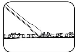
With the rear of the tooth firmly located, lock the clamping lever, and repeat the cutting test. If the sharpening wheel is not grinding a sufficient amount off the face of the tooth, repeat the above adjustment but rotate the chain stop adjustment knob clockwise.
