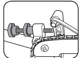
Once sharpening of the tooth completed, rotate the guide clamp lever fully to the left to unlock the chain clamp (sliding guide).
