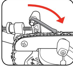
2. Adjust the chain stop so that it is firmly behind and at the bottom of the aligned chain tooth by rotating the chain stop adjustment knob either clockwise to move the chain stop forward or anti-clockwise to move the chain stop backward.
