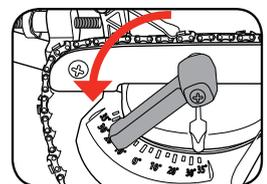
Slide the chain to the right, allowing the chain stop to ride over the links and teeth until the next tooth (orientated the same as the first tooth) rides under the stop.
