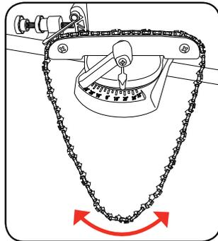
3. If you know the angle of the chain, rotate the table to the same angle as the chain. To rotate the table loosen the table lock knob and rotate the table until the scale indicator lines up with the scale on the base of the sharpener.
