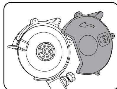
4. Hold the wheel with one hand and using the free hand turn the knob at the centre of the wheel anti clockwise. Remove the knob.
