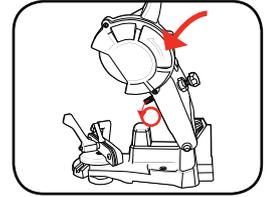
5. Whilst still applying downward pressure on the hand piece simultaneously start rotating the depth adjustment knob anti clockwise. Slowly continue rotating the knob anti clockwise whilst watching the sharpening wheel get closer to the tooth of the chain.
