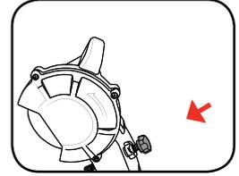
3. Rotate the lock knob towards the housing of the tool.
