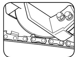
**DO NOT** attempt to try and make a heavy pass. It should be a very light "brush" of the front face of the tooth. If the cut is too heavy, stop and allow the hand-piece to rise back up, and turn the tool off. If the pass was too heavy, adjust the chain stop adjusting knob in an anti-clockwise direction slightly (suggest no more than 1/8 of a turn). Then tighten the chain stop adjusting knob lock nut.
