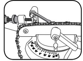
2. Rotate the depth adjustment knob clockwise as far as it will go (so as much of the pin is exposed under the head piece as possible).
