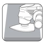
**Note:** Do not apply heavy pressure to the tool or tilt the sanding base as this will wear out the sanding paper and may damage the sanding pad.
