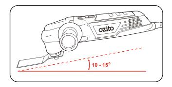
Allow the scraper to do the work; do not apply heavy pressure to the multi function tool. This may cause the multi function tool to overload or cut into the surface of the workpiece.
