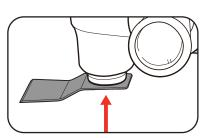
Note: Ensure the accessory is sitting flat on spindle and locking pins.
