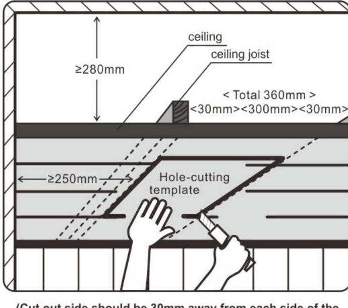
(Cut out side should be 30mm away from each side of the ceiling joist or other obstructions)
