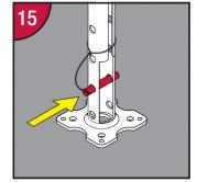
AS SOON AS THE HYDRAULIC WARNING OPERATION HAS BEEN COMPLETED, THE MECHANICAL COLLAR AND PIN FUNCTION MUST BE ENGAGED IMMEDIATELY TO AVOID THE POTENTIAL FOR ACCIDENT/DAMAGE.
