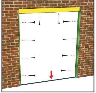
**STEP. 5.**Secure door inside opening using screws provided.
