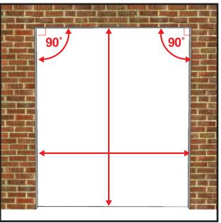
**STEP. 1.** Measure opening width/height to ensure correct size requirements.
