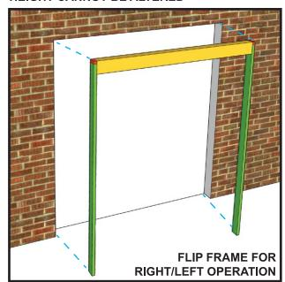
**STEP. 4.**Position constructed frame into door opening ensuring frame is square and level.
