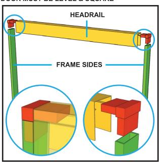
**STEP. 3.**Construct door frame by connecting Headrail to frame sides using corner pieces provided.
