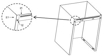
Slightly widen the two sides of the flue and hook them onto the hood body, making sure that
