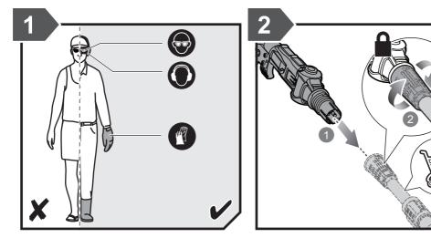
Wear full eye and head protection while operating the product. When handling the blade assembly, wear non-slip, heavy-duty protective gloves. Wear non-skid, protective footwear that will protect your feet and improve your footing on slippery surfaces.
