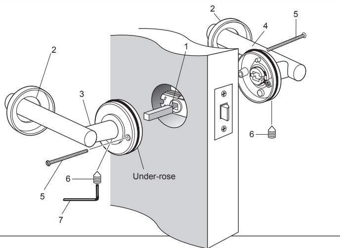
**NOTE:** Carefully follow these instructions when installing. Screws to be tightened to a recommended 2.5Nm torque.
