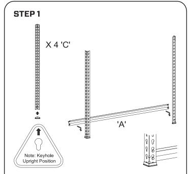
Place foot end caps onto the bottom of the 4 legs 'C'. Note upright position. Place shelving bracket 'A' onto the legs 'C'. A rubber mallet can be used to lightly tap all brackets into the key holes of the legs into place.
