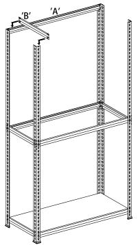
Fix Brackets 'A' at the very top allowing enough room for the MDF Shelf to sit against the legs. Repeat with Brackets 'B'.
