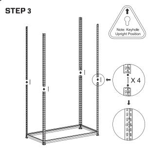
Place MDF board on bottom shelf to minimise buckling. Join the upper legs to the lower legs with the connector pins. Note upright position. Note: The legs are designed to sit directly on top of each other – don't overlap them. Handy Hint: Flathead screwdriver may be used to tap in connector pins.
