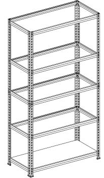
Apply remaining Brackets as above to desired height.
