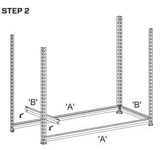
Use Shelf Brackets 'B' for the side brackets, using the Shelf Bracket from Step 1 as a guide for height.
