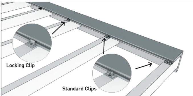
2. Screw down the clips ensuring they are tight and secure. You only need one screw per clip.
