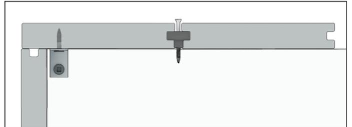
3. Repeat these steps and lay approximately 6-10 boards before screwing down properly (this is a guide only). Measure out from the 1st board to the last board to ensure that the boards are square.
