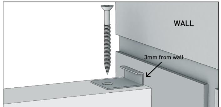
2. Run a string or chalk line from the front edge of the C-Clip between the first and last C-Clip and mark the remaining joists.
