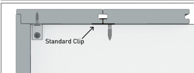
3. Gently push the next Ekodeck+ board into the clips, you may need to use a rubber mallet to seat the boards firmly in the clips.
