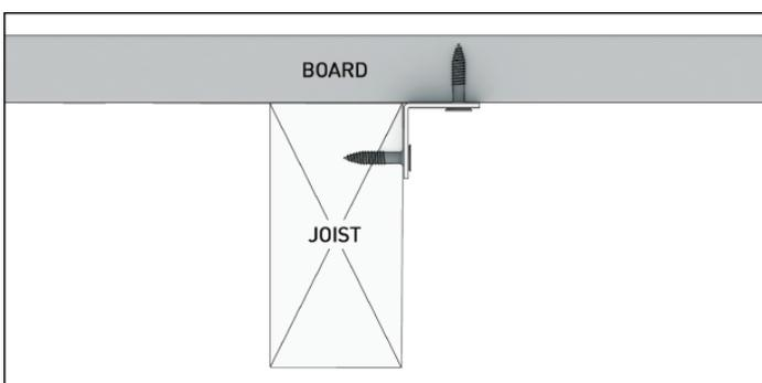
3. You can now begin to fasten your boards using Standard and Locking Clips – refer to Fastening Boards section.
