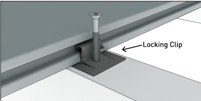
Ensure you have installed 1 (one) Locking Clip per board. Failing to install a Locking Clip will allow your boards to shift and come out of alignment.
