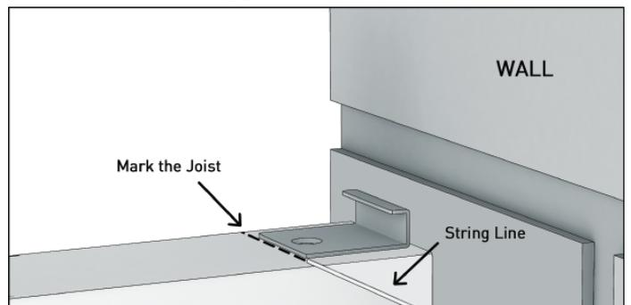
3. With the top of the joists now marked, install the rest of the C-Clips. C-Clips can be placed on every second joist if necessary. Gently push the first Ekodeck+ board into the C-Clips. You may need to angle the board slightly to push into the C-Clips.
