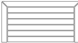
Example of a breaker board design (recommended for decks longer than 5.4m):
