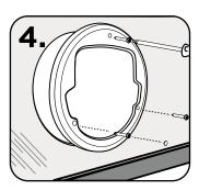
4. Ensure door is level and secure using the screws provided. Cover screws with screw covers.
