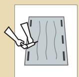
2. Place recommended double sided mounting tape and recommended adhesive (see below) in long even strips to rear of splashback.
