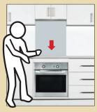
**3.** Place splashback on spacers. Press splashback firmly onto wall and make final adjustment.
