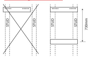
Bracket must be fastened securely at both ends. Fit timber battens to span wall studs if required.
