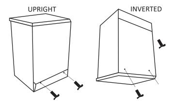
Remove indicated screws on dryer and fit plastic spacer legs with 8gx25mm screws as supplied with kit.
