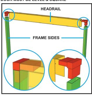
**STEP. 3.**Construct door frame by connecting Headrail to frame sides using corner pieces provided.
