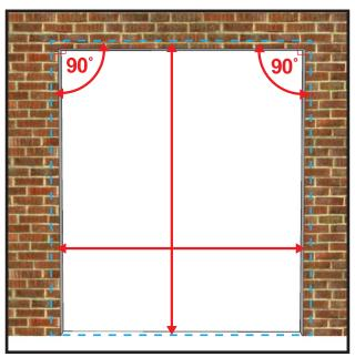
**STEP. 1.** Measure width/height to ensure correct size requirements.
