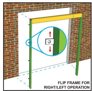
**STEP. 4.**Place face-mount brackets in desired locations and position constructed frame over door opening ensuring frame is square and level.
