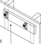
need to fit a 75x20mm timber batten as shown above and attach the brackets to the batten.
