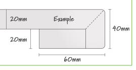
40mm edge profile comprise mitred 2 pieces of 20mm stone laminated together on visible edges only
