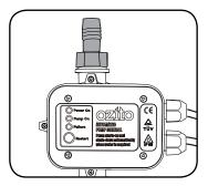
Securely attach the output hose or pipe (not included) to the other end of the adaptor. Ensure you have the correct diameter hose or pipe that is compatible with your water discharge application.
