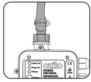
**Note:** The discharge hose or pipe you are using must have a minimum diameter of 19mm (3/4").
