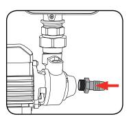
Securely attach the input hose or pipe (not included) to the other end of the adaptor. Ensure you have the correct diameter hose or pipe that is compatible with your water drawing source and pump.
