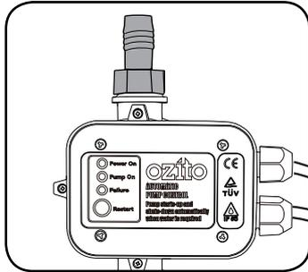
2. Securely attach the output hose or pipe (not included) to the other end of the adaptor. Ensure you have the correct diameter hose or pipe that is compatible with your water discharge application.
