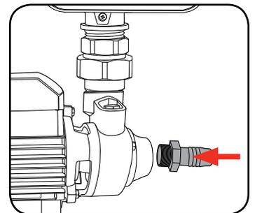
2. Securely attach the input hose or pipe (not included) to the other end of the adaptor. Ensure you have the correct diameter hose or pipe that is compatible with your water drawing source and pump.
